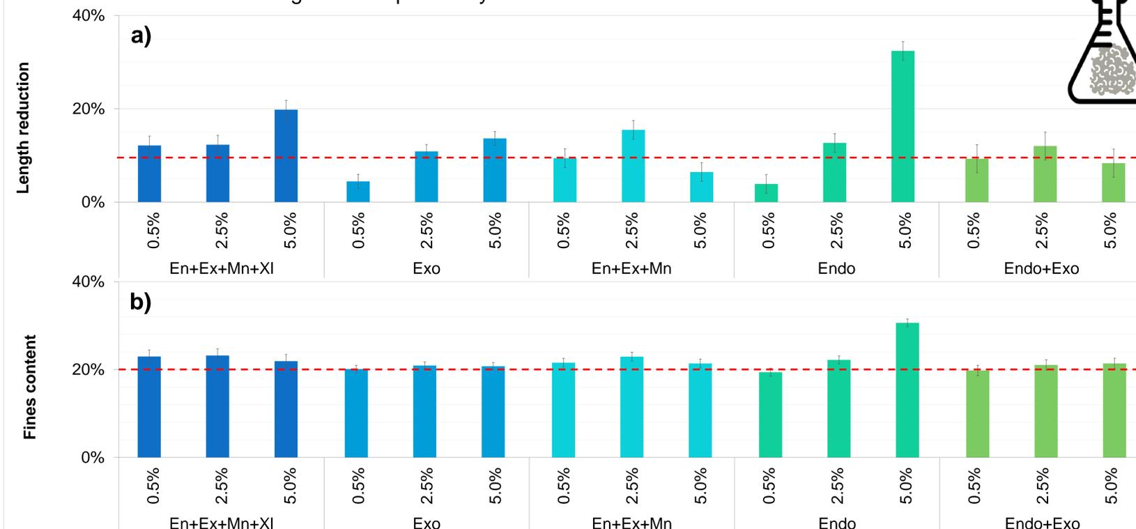
Fig. 2 Effect of enzyme type and dosage variation on a) fibre length reduction relative to untreated fibres, and b) fines content measured on FQA. Red dashed line indicates the result of refining without enzymatic hydrolysis.
