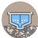
Small solid particles settle out in a **clarifier** after flocculation. Wastewater is recovered by a **belt press**.
