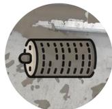
Liquid effluent from the clarifier is processed by a **rotary drum filter** to remove remaining fine solids.
